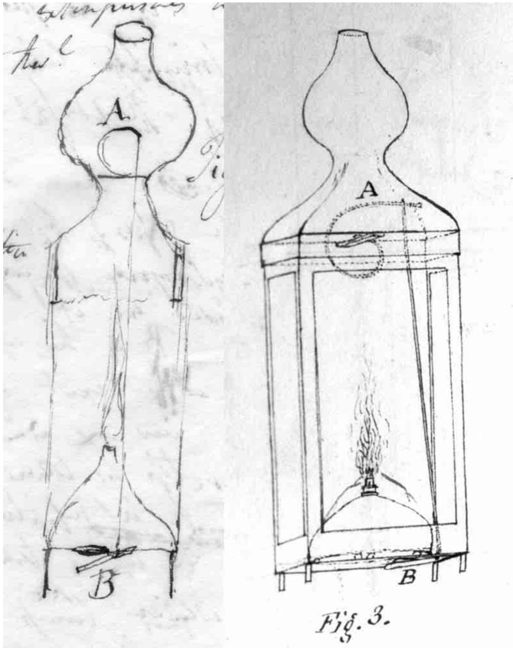
Fig. 7. Davy's lamp with the valve at the bottom. (a) Davy's sketch (RI MS HD 11, p.108) and (b) as drawn by Faraday (RS MS PT 10.1bis, p. 20).
