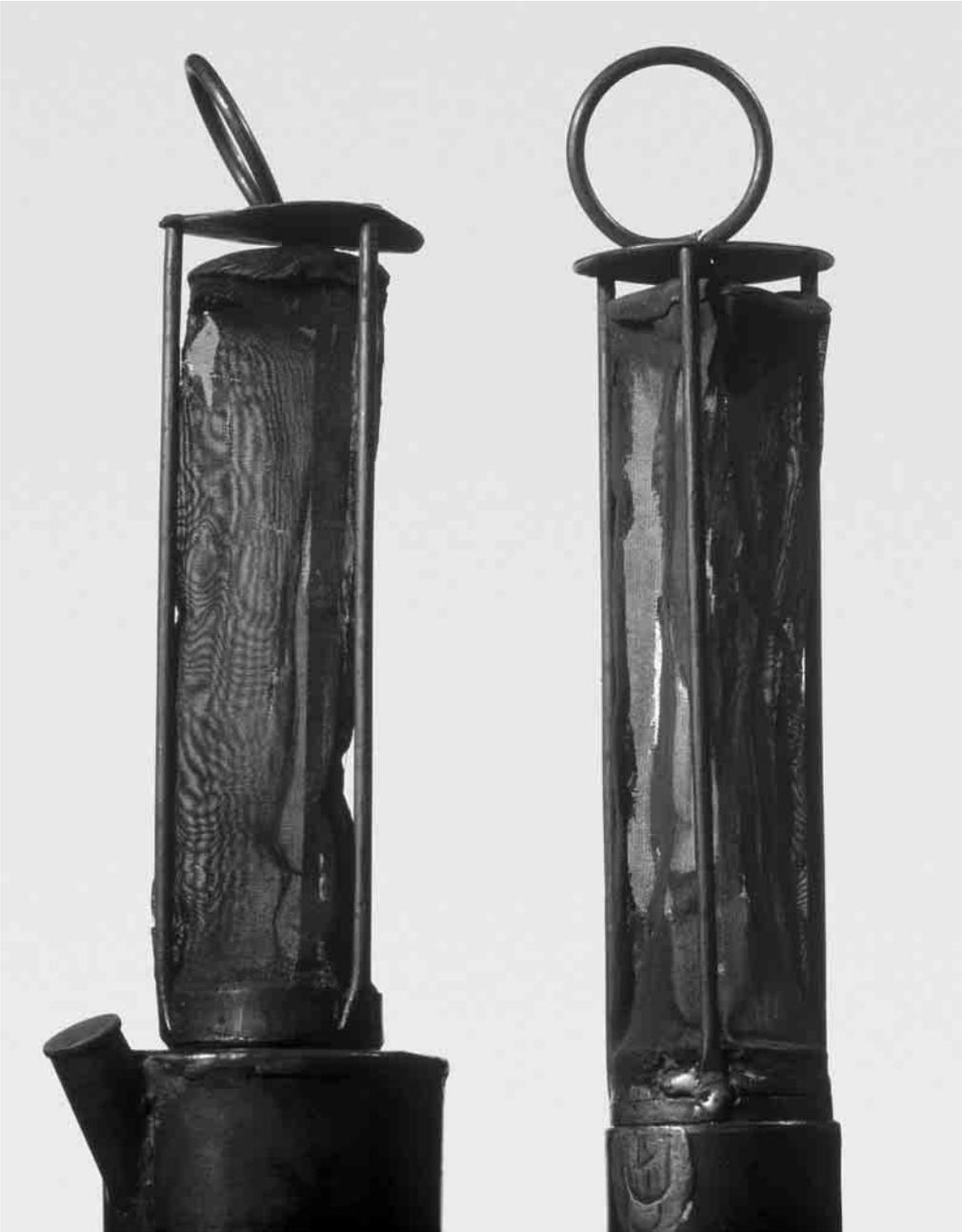
Fig. 21. Davy's gauze lamps tested in Hebburn Colliery on 9 January 1816. (NMSI Inv 1857–208).
