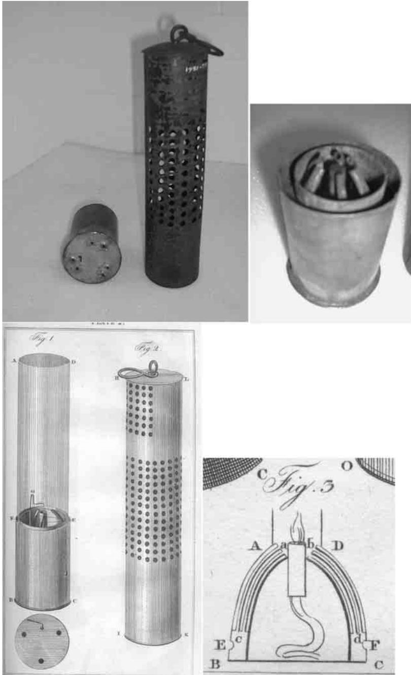
Fig. 24. Stephenson's second lamp (a) with detail (b) of inlet tubes in the Collections of the Royal Institution and (c, d) as illustrated in *Report upon the Claims of Mr. George Stephenson, relative to the Invention of His Safety Lamp* (Newcastle, 1817), opposite pp. [27] and [28] respectively.
