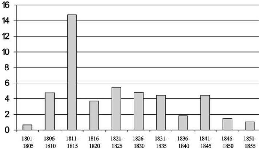
Fig. 30. Annual facilities in the North East Coal Field Period per Million Tons of Coal Produced averaged over five-year periods. Source: Combining interpolated data in Fig. 28 with data in Fig. 29.
