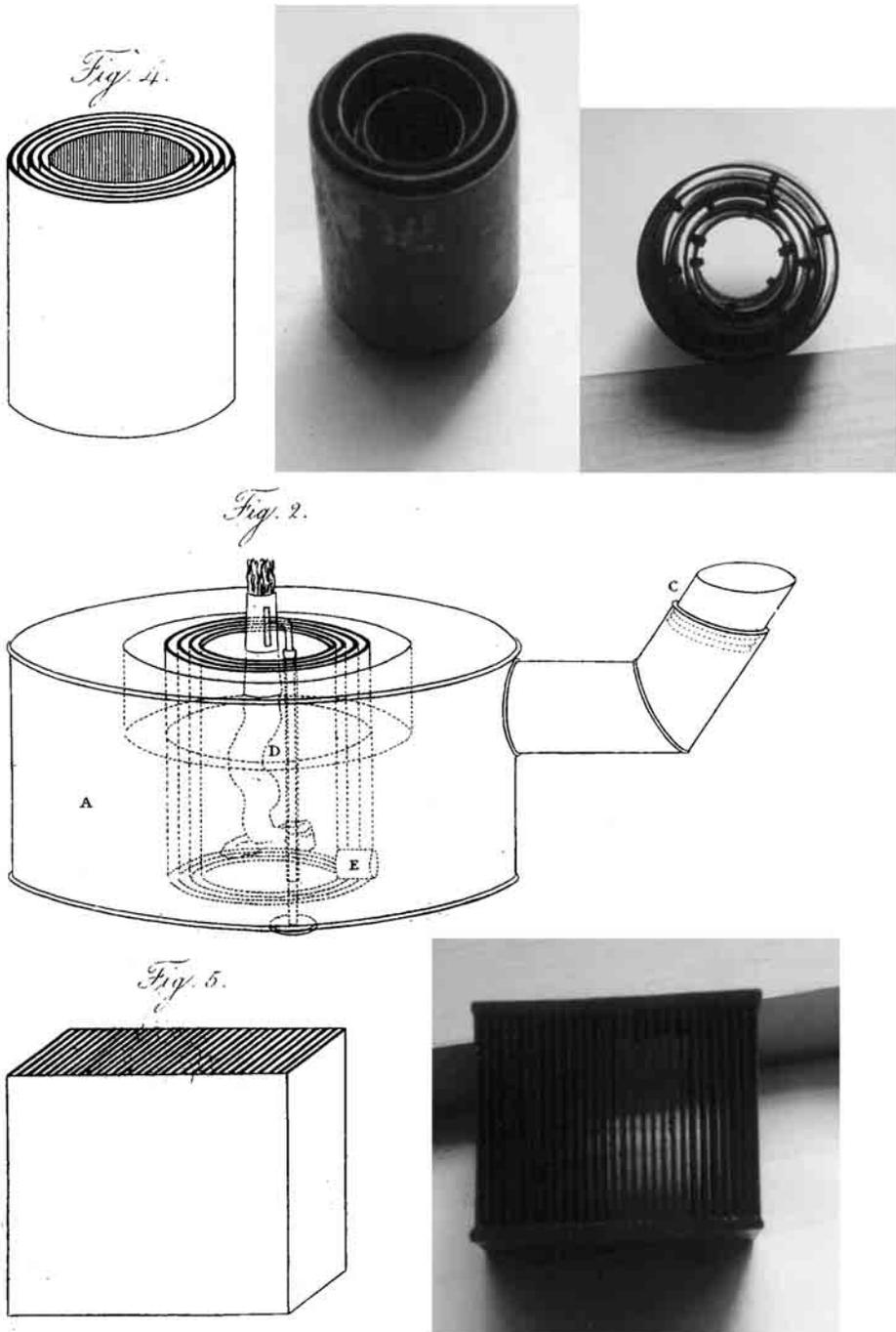
Fig. 15. (a) Drawing of Davy's circular fire sieve, (b, c) photographs of surviving example, (d) how the sieve was inserted in the base of a lamp (see also Figure 3b), (e) Davy's rectangular fire sieve, (f) photograph of surviving example. All illustrations from *Philosophical Transactions*, 106 (1816), opposite p. 22 and objects from the Collections of the Royal Institution.
