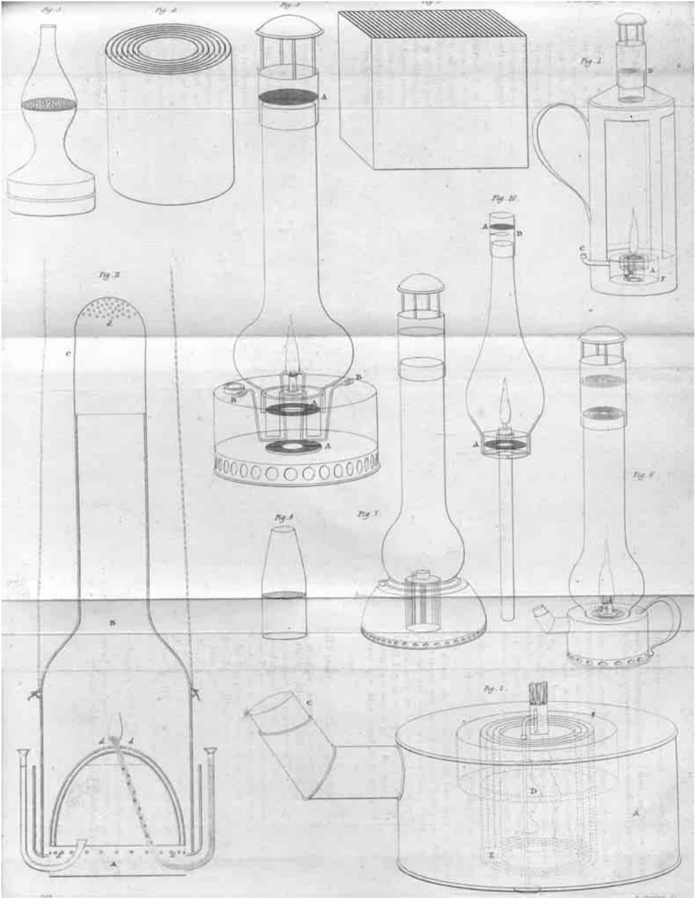
Fig. 27. Plate from *Philosophical Magazine*, 46 (1815), opposite p. 456 showing Stephenson's fourth lamp (bottom left) with the illustrations for Davy's paper.
