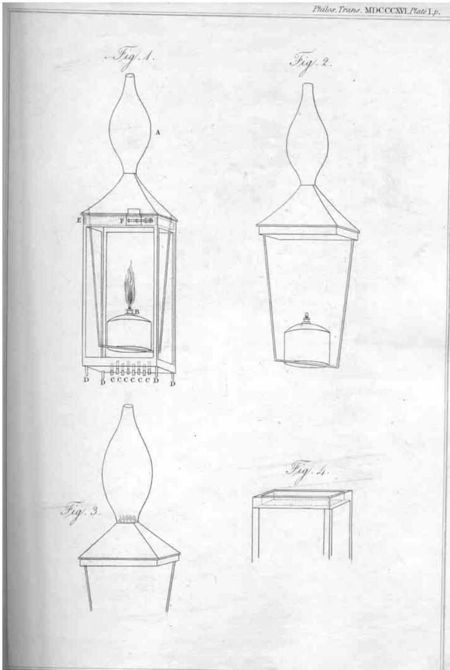
Fig. 14. First engraved plate for Davy's paper. This is in RI MS HD 11, p. 115 and is the only copy so far located.
