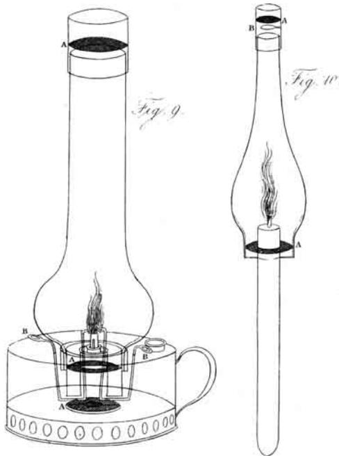
Fig. 18. Davy's method of using gauze to protect (a) an ordinary lamp and (b) a candle lamp. From *Philosophical Transactions*, 106 (1816), opposite p. 22.
