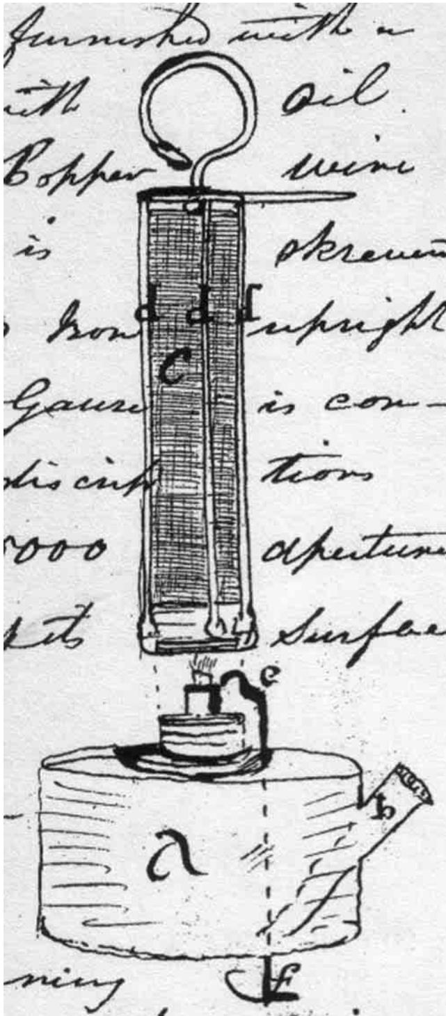
Fig. 22. Matthias Dunn's drawing of a Davy gauze lamp tested at Hebburn Colliery on 9 January 1816. (From NEOAMB MS 1997-202, p. 24).
