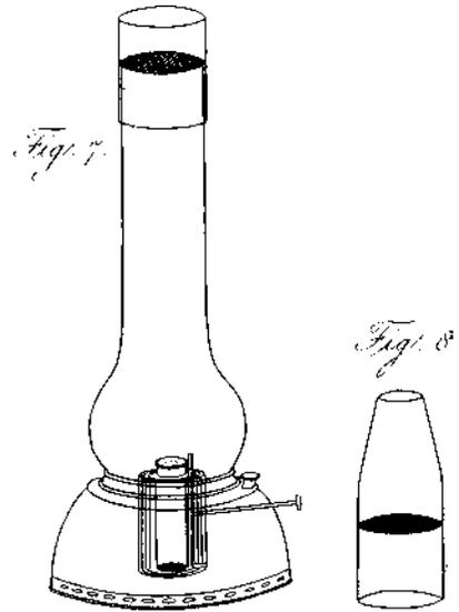
Fig. 17 (above right). Davy's method of protecting an Argand Lamp by using a chimney with a metallic gauze insert (detail). From *Philosophical Transactions*, 106 (1816), opposite p. 22.
