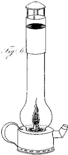
Fig. 16 (above left). Glass lamp rendered safe by use of a concentric fire sieve in chimney. From *Philosophical Transactions*, 106(1816), opposite p. 22.
