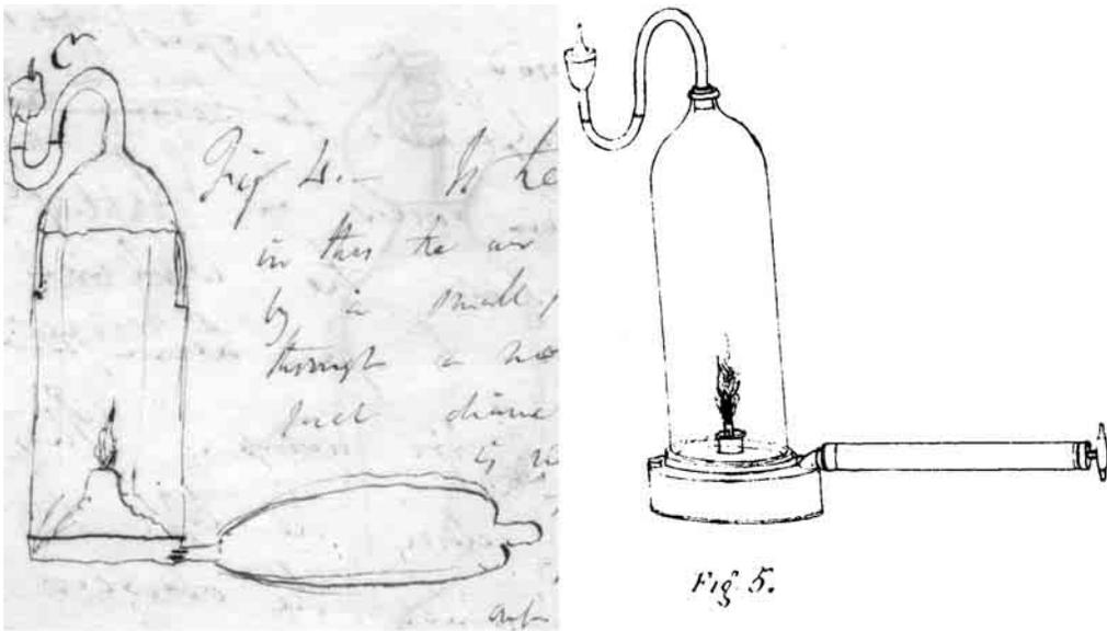
Fig. 8. Davy's bellows lamp. (a) Davy's sketch (RI MS HD 11, p. 108) and (b) as drawn by Faraday (RS MS PT 10.1bis, p. 20).
