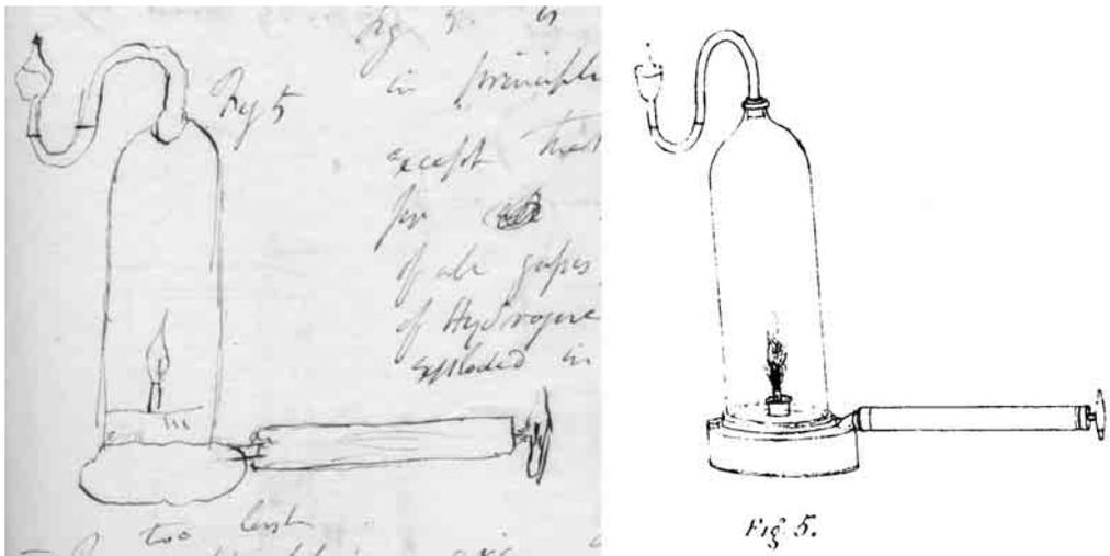
Fig. 9. Davy's piston lamp. (a) Davy's sketch (RI MS HD 11, p. 109) and (b) as drawn by Faraday (RS MS PT 10.1bis, p. 21).
