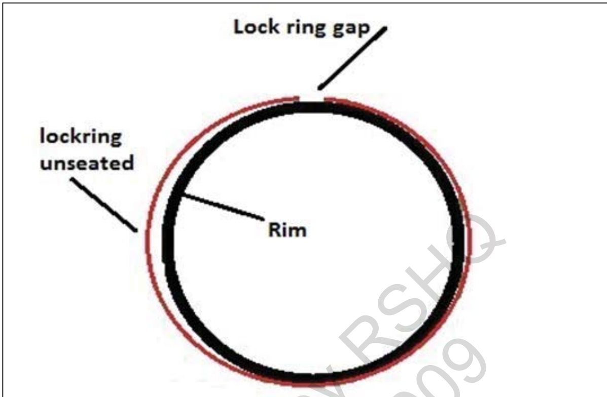
Figure 36: Diagram showing an open lock ring (excessive gap end).
