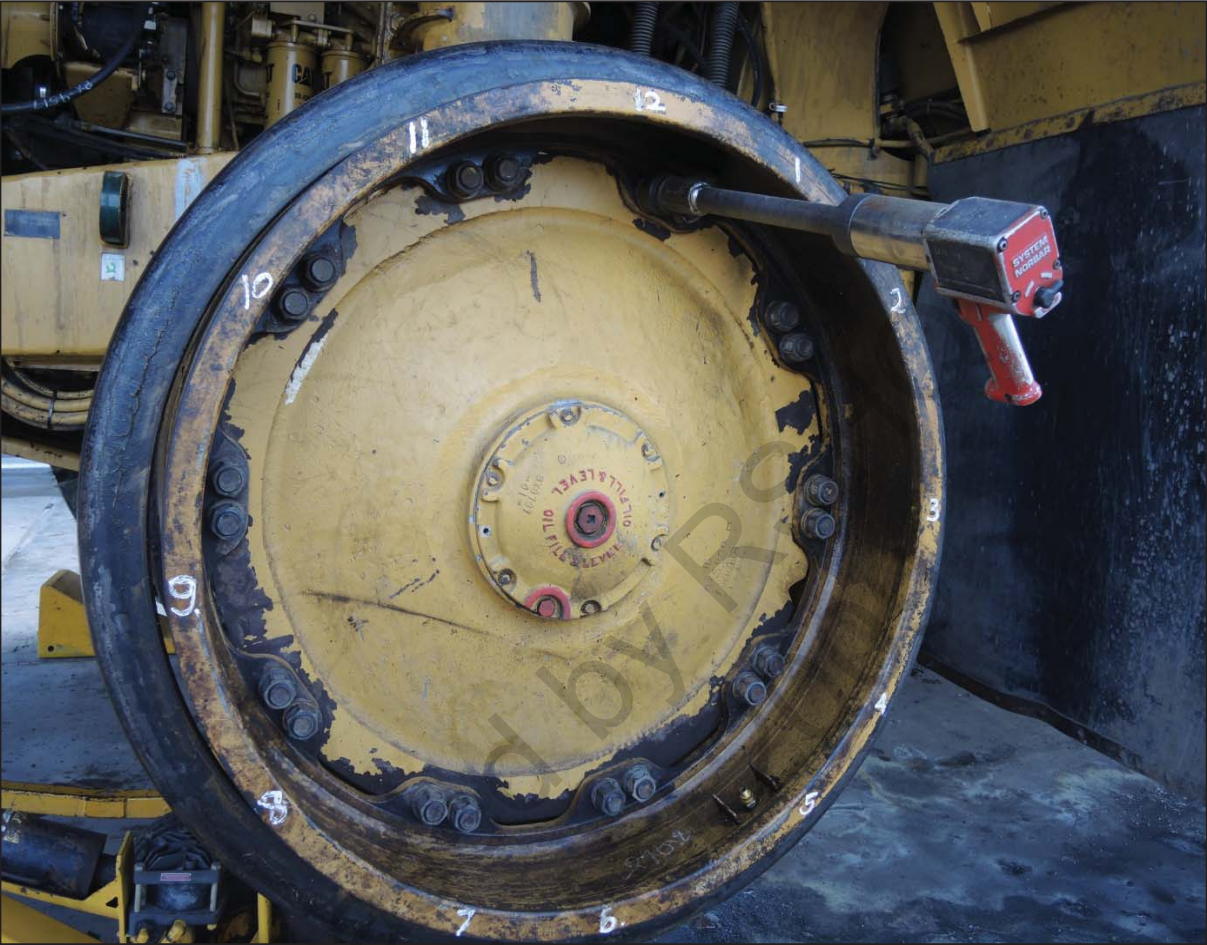
Figure 35: Five nuts at location numbers 2 to 6 (from DNRM photos taken at incident scene).
