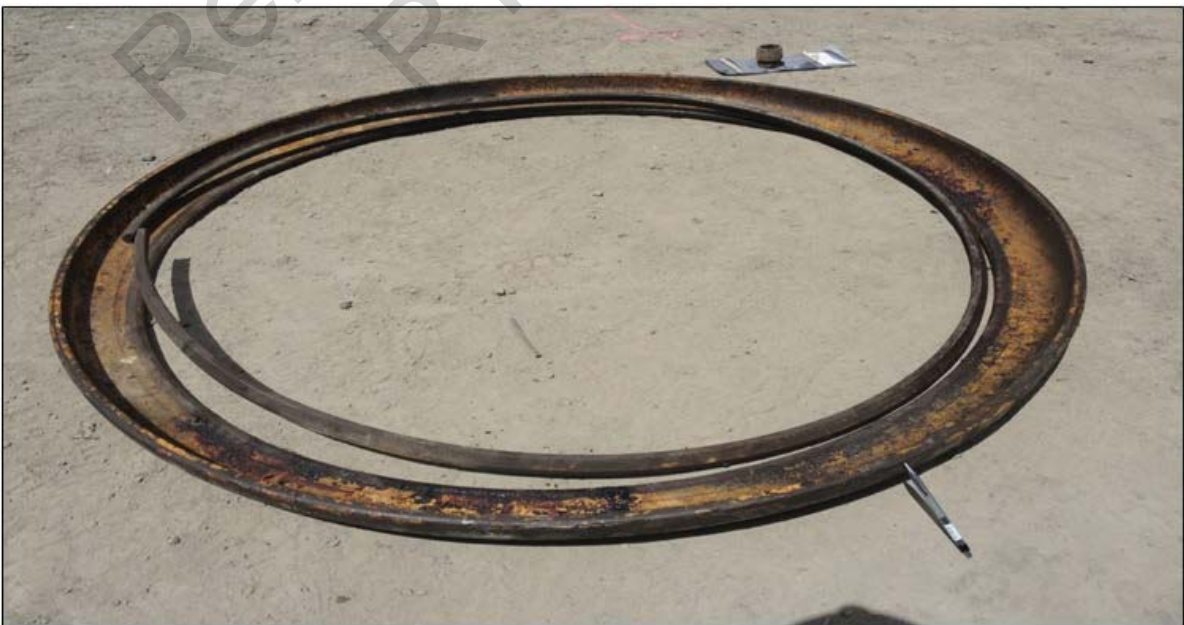
Figure 40: Distinctive spiral shape of lock ring (from DNRM photos taken at incident scene).
