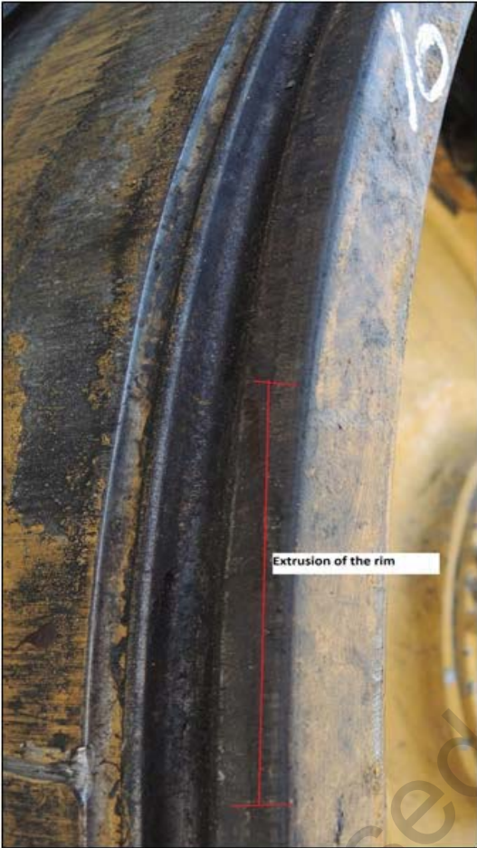
Figure 38 and 39: Extrusion of rim (from DNRM photos taken at incident scene).
