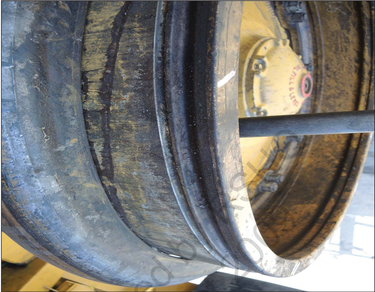
Figure 16: Standard of cleaning of rim (from DNRM photos taken at incident scene).
