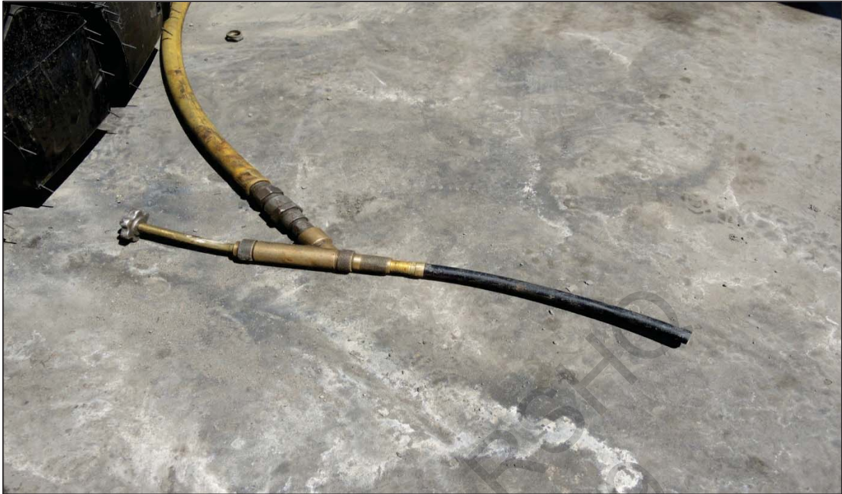
Figure 26: Part of the valve stem (from DNRM photos taken at incident scene).
