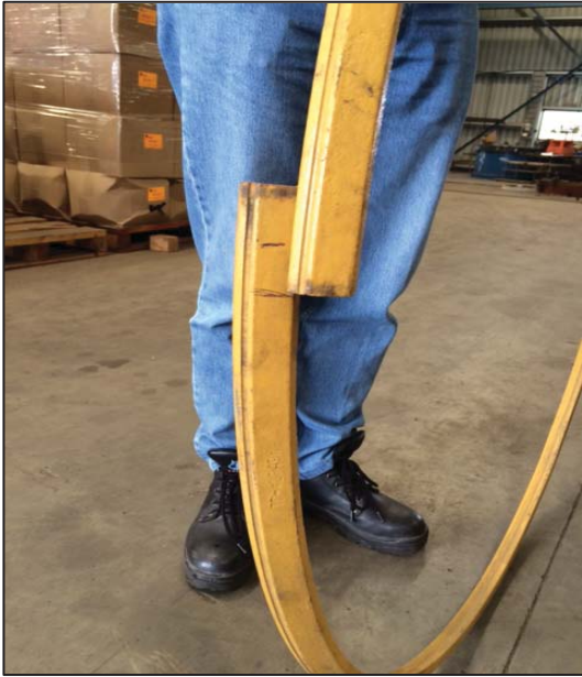
Figure 10: 49 inch EV lock ring end overlap of 50mm measured at the 9 o'clock position (taken by DNRM Inspectors at Rimex Mackay).
