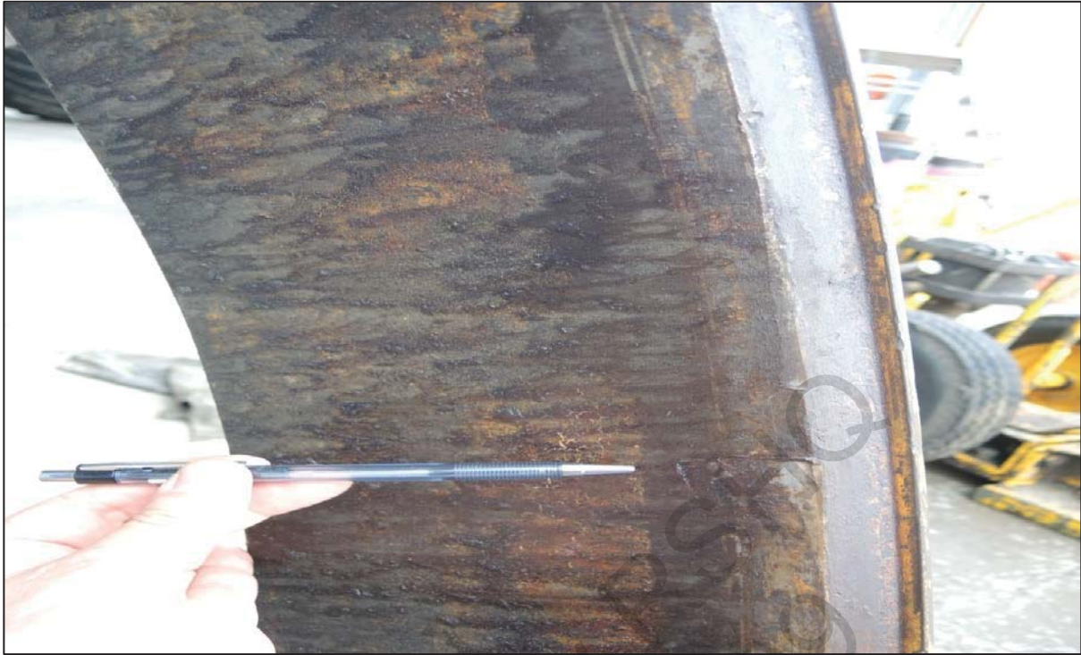
Figure 21: Witness marks that occurred during the peeling of the lock ring (from DNRM photos taken at incident scene).
