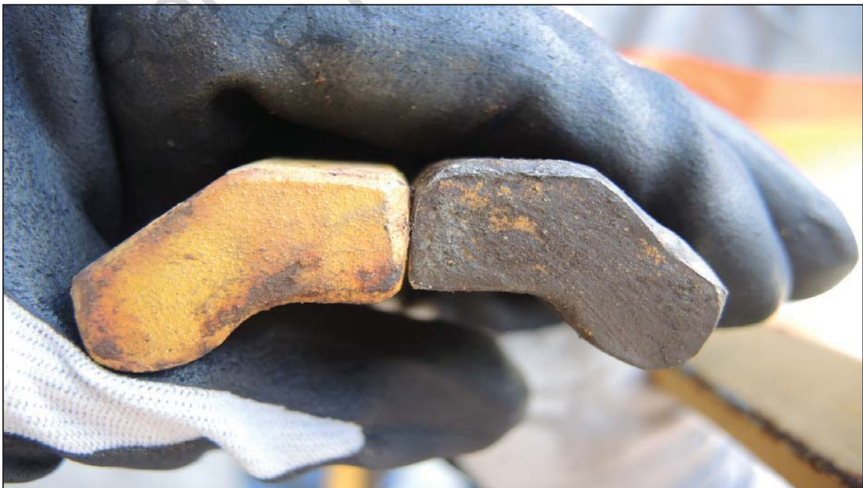
Figure 18: Profile comparison to a new lock ring of the same part number (from DNRM photos taken at incident scene).
