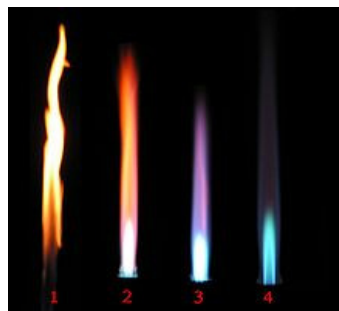
Figure 8.3 Various types of flame from a Bunsen burner
