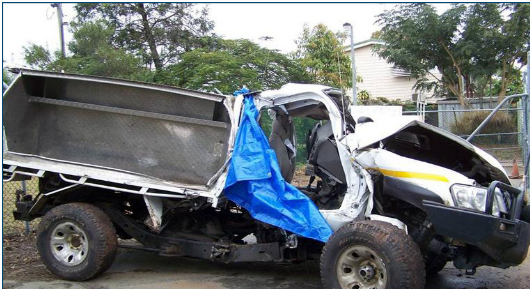
Picture 8: Right hand side of utility showing toolbox mounted to the tray.
