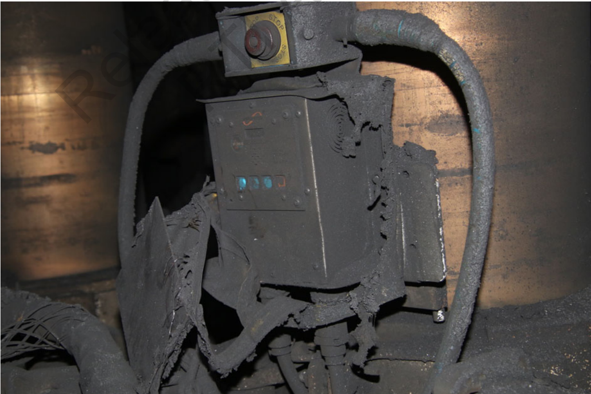
Images 15 – 17 Increasing fire damage in surfaces from Chocks 107 to 110
