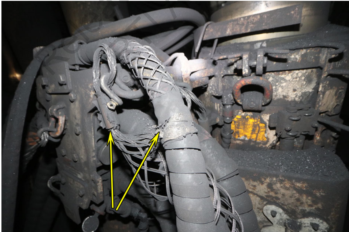
Images 12 – 14 Limited damage to fixtures at Chock 100 (above) with slight damage observed at some surfaces at the adjacent Chock 101
