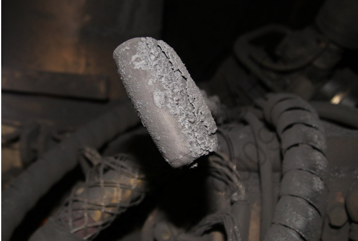
Image 27 Ignited coal dust has condensed onto the side of surfaces by passing ventilation
