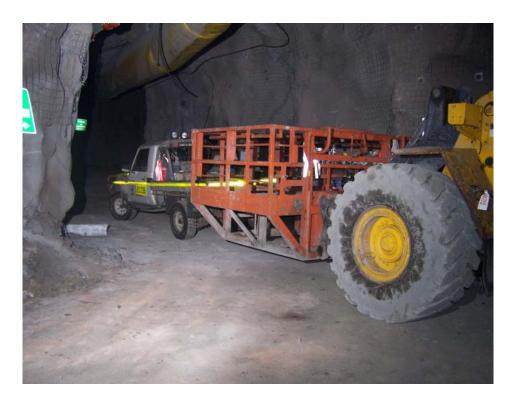
The loader with the attached work platform positioned adjacent to the rear tray of the Landcruiser
