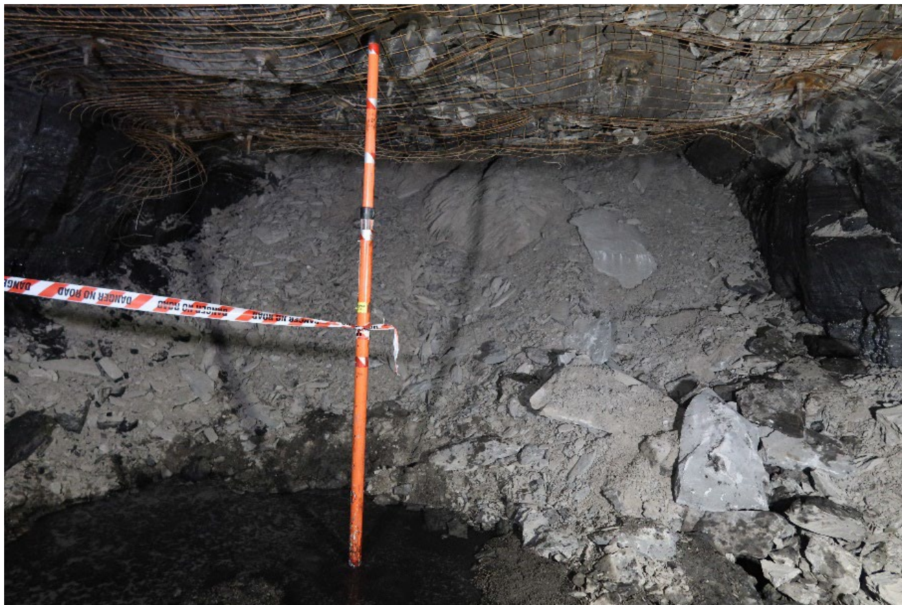
Figure 3: The void above the coalface in Razorback Mains B heading 11-12 cut-through
