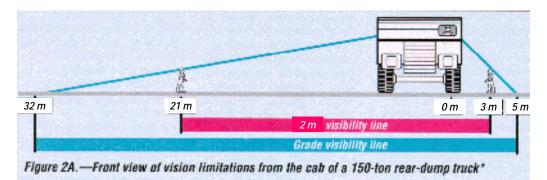
Illustration of blind spots around a mining truck (from Miller, 1975)<sup>2</sup> Illustration indicative of vision from a large RDT, distances shown are approximate.
