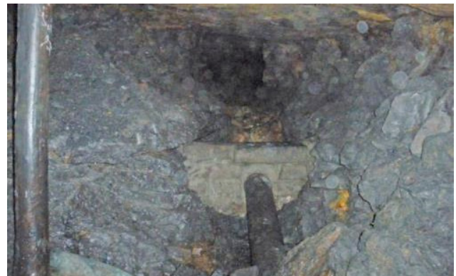
Figure 9 The dam and black pipe at the Lower Monks on the Main Drift
