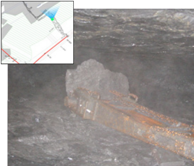
Figure 14 The top end of the armoured face conveyor that had been driven back about 4 m by the force of the water
