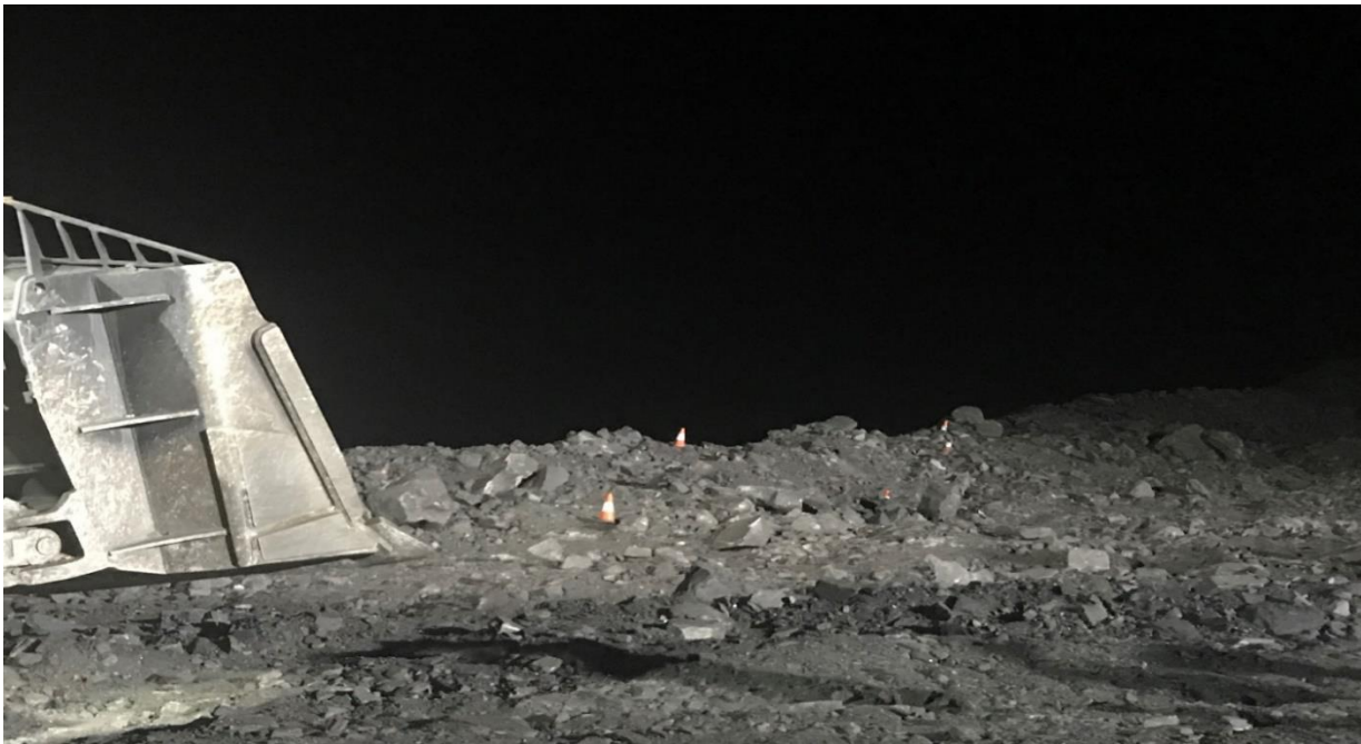
Photograph of area where dozer 804 drove over edge showing lighting.
