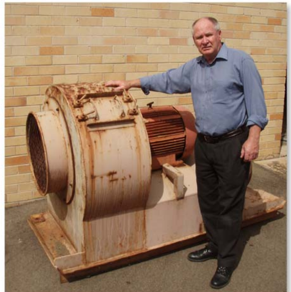
TestSafe's Bill Dunn with the electric powered fan which he found in his 1979 investigation to be the cause of ignition for the Appin Mine Explosion
